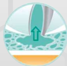
Figure 3: As soon as the sharp object breaks through, it is enveloped by the solution and the viruses or bacteria are effectively neutralised.
